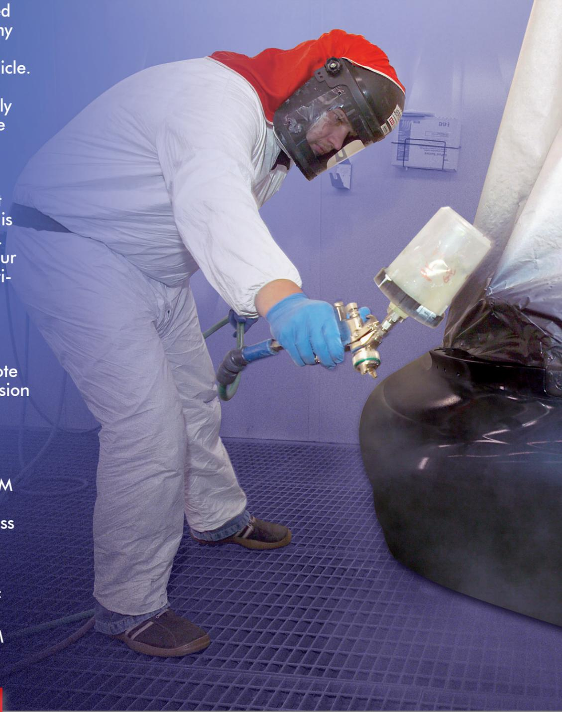
**Different application processes and substrates can result in colour variation on plastic bumpers compared to metal body parts.**
